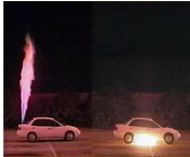
Ignition of both fuels occur. Hydrogen flow rate 2100 SCFM (0.18 m 3 /min.) Gasoline flow rate 680 cm 3 /min.
