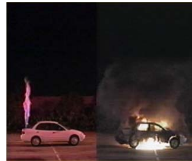
Hydrogen flow is subsiding, view of gasoline vehicle begins to enlarge
