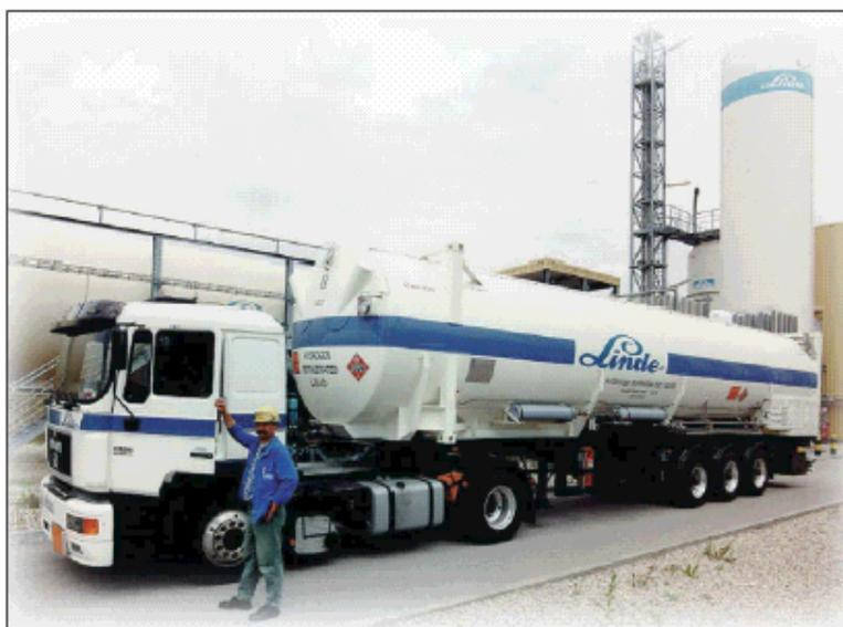
Fig. IX.9: Trailer for liquid  $\text{H}_2$  transport (total weight 40 tons; load 3370 kg)
