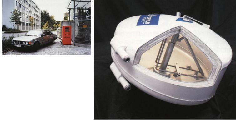
Fig. IX.10: BMW 745i refilled with liquid hydrogen (left photograph). Exploded view of the liquid hydrogen tank (right panel).
