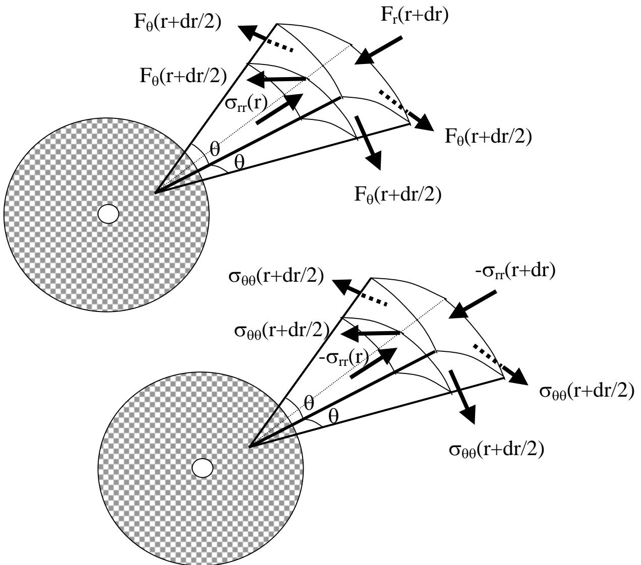
**Fig.A. IV.3:** A spherical sample with a central hole at pressure  $p$ . The net force on each volume element must be zero (top panel). The bottom panel shows the corresponding stresses. The negative signs are due to the choice of positive stresses in Fig.A. IV.2. This determines a differential equation for the stresses (see Eq.A.IV.7).
