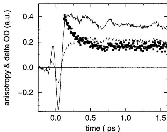
**Figure 5.** The 5 K anisotropy measurement. Excitation was at 1055 nm and detection at 1070 nm; shown are the parallel (solid), perpendicular (dash) pump-probe response, the calculated (squares) and the fitted anisotropy (solid). The anisotropy was fitted with a 150 fs monoexponential decay and a remaining anisotropy of 0.16.
