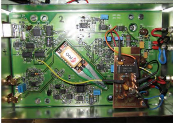
Figure 3.3: Low noise, high modulation-bandwidth laser-driver electronics including temperature stabilisation, developed in house at VU Bèta Elektronica. The Rio Planex laser diode is clearly visible in the middle as the rectangular electronics package marked RIO. Note that the electronics are built into an EMI enclosure and that filtered feed-throughs (right side, with the red leads soldered on) are used to connect the power supplies.
