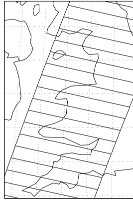
Figure 3.2: GOME ground surface pixel coverage (solid boxes) of about 0.4^\circ \times 4^\circ shown along with the 1^\circ -grid size of the ECMWF assimilation model (dotted grid).
