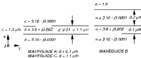
Figure 1 Waveguide geometries. The left waveguide is symmetric, the right strongly asymmetric.
