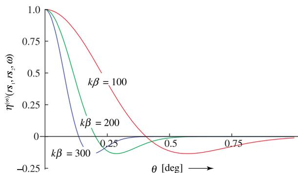
Figure 7. The spectral degree of coherence of the far field generated by a planar, unpolarized Laguerre–Gauss source. The three curves correspond to sources with different values of the parameter  $k\beta$ . (The color version of this figure is included in the online version of the journal.)
