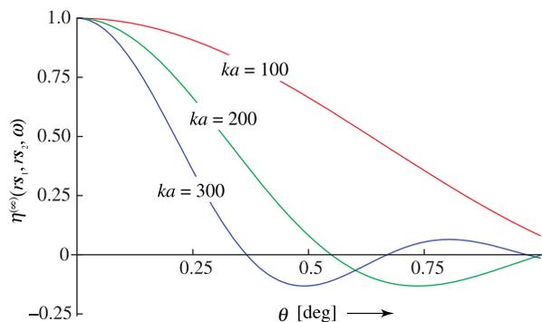
Figure 6. The spectral degree of coherence in the far zone of an unpolarized beam emerging a circular aperture. The three curves correspond to sources with different values of the normalized aperture size  $ka$ . (The color version of this figure is included in the online version of the journal.)
