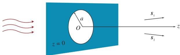
Figure 5. Notation relating to collimated blackbody radiation emerging from a circular aperture. (The color version of this figure is included in the online version of the journal.)
