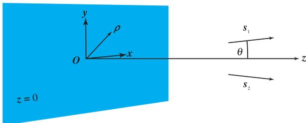
Figure 2. Notation relating to radiation generated by a planar, stochastic source. (The color version of this figure is included in the online version of the journal.)
