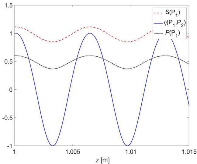
**Fig. 2.** The spectral degree of coherence  $\eta(P_1, P_2)$  (solid blue curve), together with the scaled spectral density (red dashed) and the degree of polarization (black dotted) at the observation points as a function of the distance  $z$ . In this example  $\delta_{xx} = 1$  cm,  $\delta_{xy} = 1.41$  cm,  $B_{xy} = 0.5$ ,  $\lambda = 632.8$  nm,  $d = 1$  cm, and  $s = 5$  mm. Hence  $\mu = 0.135$  and  $\mu_{xy} = 0.365$ .
