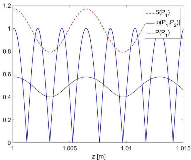
**Fig. 3.** The modulus of the spectral degree of coherence  $\eta(P_1, P_2)$  (solid blue curve), together with the scaled spectral density (red dashed) and the degree of polarization (black dotted) for two asymmetric observation points  $P_1 = (s, 0, z)$  and  $P_2 = (-2s, 0, z)$ , as a function of the propagation distance  $z$ . In this example  $\delta_{xx} = 1$  cm,  $\delta_{yy} = 1.2$  cm,  $\delta_{xy} = 1.41$  cm,  $B_{xy} = 0.5$ ,  $\lambda = 632.8$  nm,  $d = 1$  cm, and  $s = 5$  mm.
