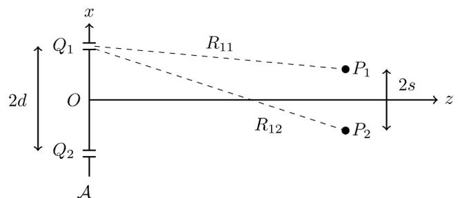
Fig. 1. The superposition of the fields radiated by two identical pinholes at  $Q_1$  and  $Q_2$  in a screen  $\mathcal{A}$  is observed at two symmetrically located positions  $P_1$  and  $P_2$ . The origin  $O$  is located midway between the apertures.  $R_{11} = |Q_1 P_1|$ , and  $R_{12} = |Q_1 P_2|$ ;  $R_{22}$  and  $R_{21}$  are not shown. The separation between  $Q_1$  and  $Q_2$  is  $2d$ , that between  $P_1$  and  $P_2$  is  $2s$ .
