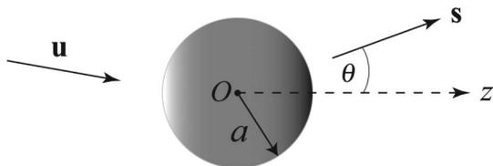
**Fig. 1.** A homogeneous sphere with radius  $a$  is illuminated by a plane wave propagating in the direction  $\mathbf{u}$ . The scattering angle  $\theta$  is the angle between the positive  $z$  axis and an observation direction  $\mathbf{s}$ . Both  $\mathbf{u}$  and  $\mathbf{s}$  are unit vectors. The point  $O$  is the origin of the coordinate system.
