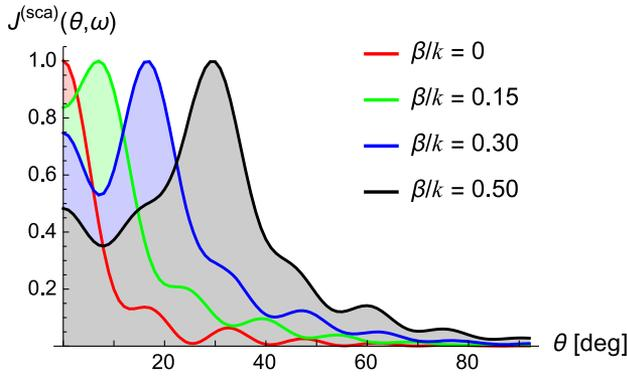
**Fig. 2.** Angular distribution of the normalized radiant intensity of the scattered field for selected values of the normalized coherence parameter  $\beta/k$ , namely: 0 (red), 0.15 (green), 0.30 (blue), and 0.50 (black). In this example, the wavelength  $\lambda = 632.8$  nm, the refractive index  $n = 1.33$ , and the sphere radius  $a = 2\lambda$ .
