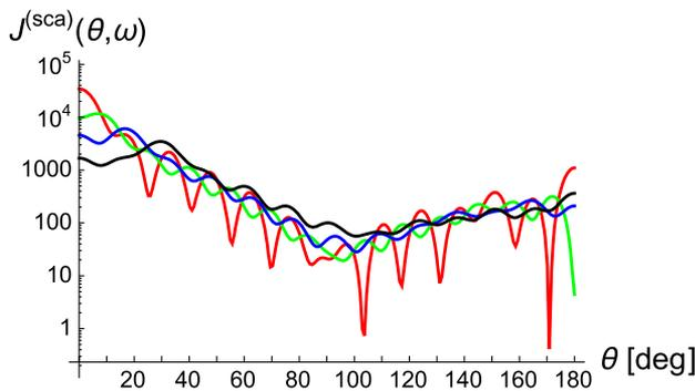
**Fig. 3.** Angular distribution of the logarithmic radiant intensity of the scattered field for selected values of the normalized coherence parameter  $\beta/k$ : 0 (red), 0.15 (green), 0.30 (blue), and 0.50 (black). The parameters are the same as in Fig. 2.
