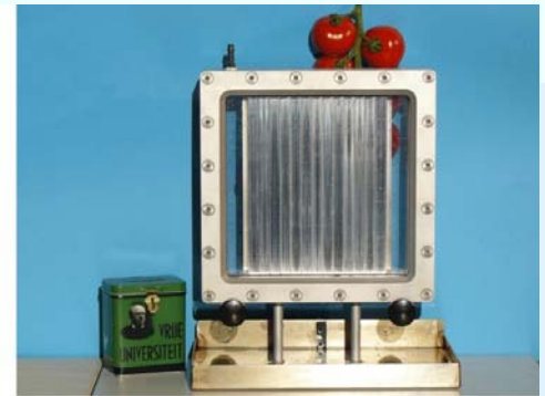
VU University developed a low-cost optical switch. The switch consists of a panel which is transparent when filled with water and light reflecting when empty.
