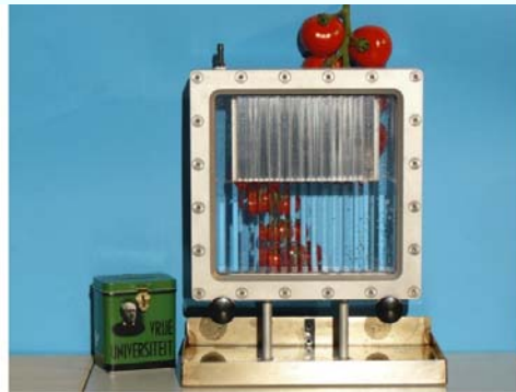
VU University developed a low-cost optical switch. The switch consists of a panel which is transparent when filled with water and light reflecting when empty.
