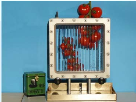
VU University developed a low-cost optical switch. The switch consists of a panel which is transparent when filled with water and light reflecting when empty.
