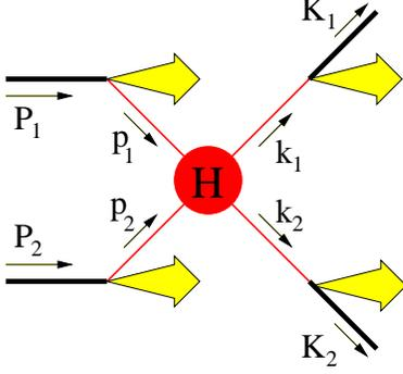
Fig. 3. – Schematic illustration of the contribution of a hard subprocess, parton ( $p_1$ ) + parton ( $p_2$ )  $\rightarrow$  parton ( $k_1$ ) + parton ( $k_2$ ), to the (2-particle inclusive) scattering process hadron ( $P_1$ ) + hadron ( $P_2$ )  $\rightarrow$  hadron ( $K_1$ ) + hadron ( $K_2$ ) + X, at the level of the amplitude. The process being hard implies for the hadronic momenta  $P_1 \cdot P_2 \sim P_1 \cdot K_1 \sim Q^2$ , etc.
