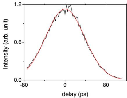
Fig. 3. Measured autocorrelation trace and Gaussian fit. The fit has a FWHM of 90 ps, which indicates a pulse length of 64 ps for a Gaussian temporal profile.
