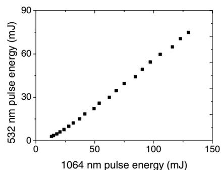
Fig. 2. Output pulse energy at 532 nm after SHG plotted against the 1064 nm input pulse energy.
