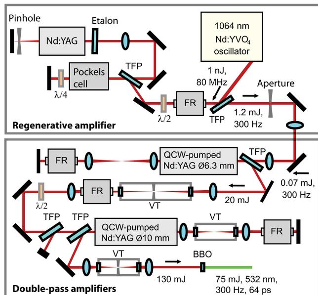
Fig. 1. Schematic of the developed Nd:YAG regenerative amplifier and quasi-CW-pumped postamplifier system. TFP, thin-film polarizer;  $\lambda/2$ , half-wave plate;  $\lambda/4$ , quarter-wave plate; FR, Faraday rotator; VT, vacuum tube.
