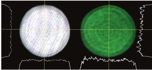
Fig. 4. Transverse beam profiles of the amplified pulses at 1064 nm (left) and after frequency doubling to 532 nm (right), measured at the position of the BBO crystal via relay imaging. Single-line cross sections at the dashed lines are included. Note that the diagonal fringes in the 1064 nm image are an artefact, due to interferences in the CCD camera. Some spots are visible in the 532 nm beam, which are caused by dust particles on neutral gray filters and the CCD itself.
