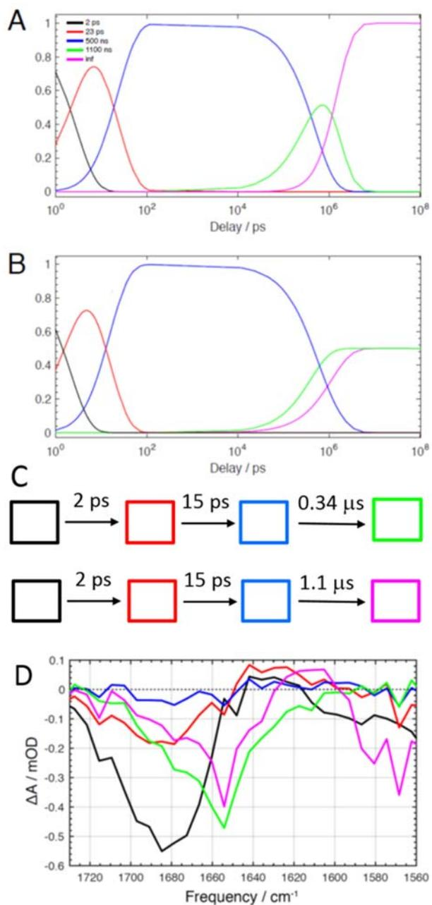
**Figure S6.** Transient concentration profiles of time-resolved IR data with sequential (A) and parallel (B) data analysis. Panel (C) shows the kinetic model for the parallel analysis. The black, red and blue compartments were assumed to have identical spectra. The population ratio between upper and lower pathway was fixed at 1:1. Panel (D) shows the species-associated difference spectra of the global analysis in terms of the kinetic model of (C).
