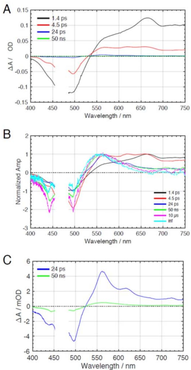
**Figure S1.** Fitting results following Global Analysis of UV-vis TA data. (A) EADS of the first 4 components; (B) EADS normalized to their respective absorption maxima; (C) 24 ps and 50 ns EADS, unscaled. Note the 1000-fold ordinate axis unit change between panel (A) and (C). The initially populated, short-lived  $S_2$  state was not resolved due to sparse sampling around time zero.
