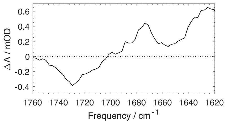
**Figure S7.** Mid-IR transient absorption spectrum of hECN dissolved in THF at a 2 ps delay. The excitation wavelength was 475 nm.
