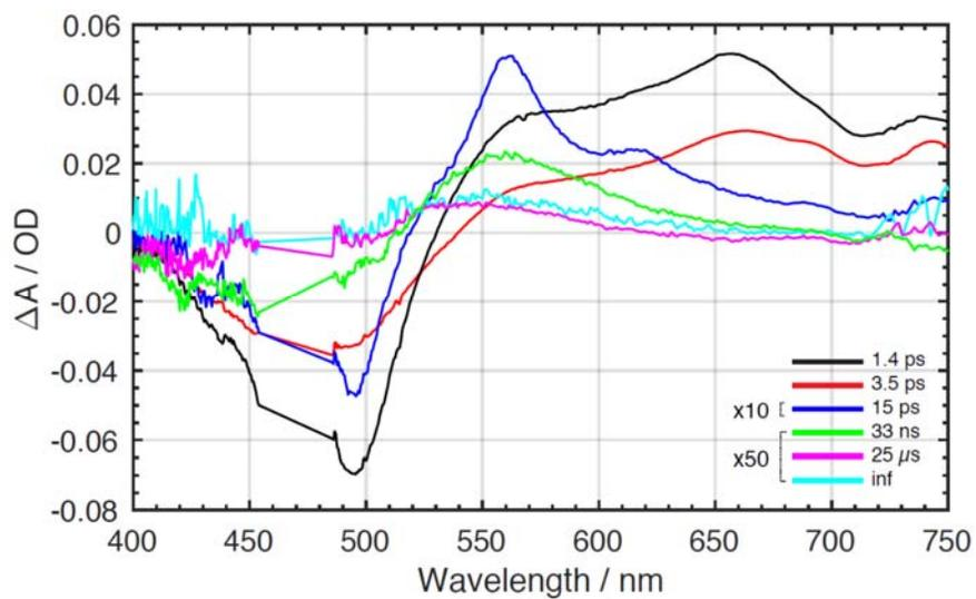
**Figure S4.** EADS of OCP at 475 nm excitation, at 150 nJ excitation pulse energy. The excitation pulse was stretched to 2 ps. The 15 ps EADS was expanded 10 times, while the 33 ns, 25  $\mu$ s and infinite EADS were expanded 50 times.
