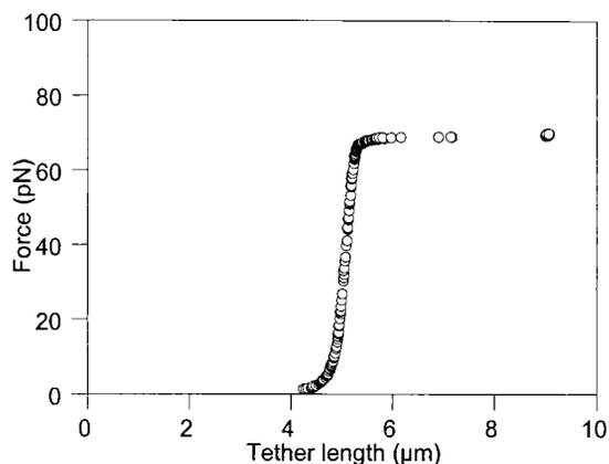
FIGURE 10 Overstretching 14,771-bp DNA with flow force. Linearized pBW8 plasmid DNA was assembled between two beads, using the automated assembly procedure. The laser-trapped bead was released from the trap and extended by flow. The DNA was stretched by ramping the flow to increase the hydrodynamic drag force.
