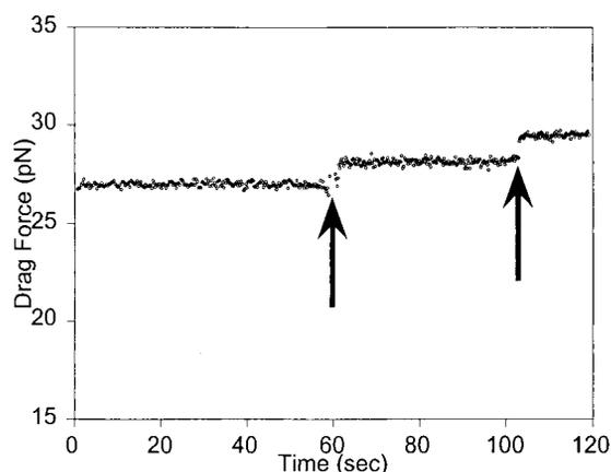
FIGURE 4 A micron-sized bead is kept in a laser trap while  $\sim 10$ -kb-long DNA molecules pass through the fluid chamber. Upon connection of a biotinylated DNA molecule to the streptavidin on the beads, the measured drag force of the bead increases ( $\uparrow$ ). This distinct increase in drag allows precise knowledge of the number of molecules attached to the bead.
