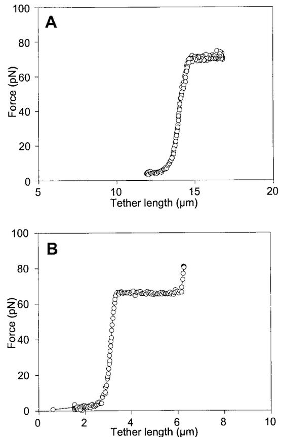
**FIGURE 9** Overstretching DNA with laser trap force. DNA was assembled between two beads, using the automated assembly procedure, and stretched by stepping the micropipette away from the laser trap. Experiments were performed in 10 mM Tris-Cl (pH 8.0), 0.5 M NaCl. (A) Bacteriophage  $\lambda$  DNA (48,502 bp). (B) *HindIII-BamHI* fragment of bacteriophage  $\lambda$  DNA (9866 bp).
