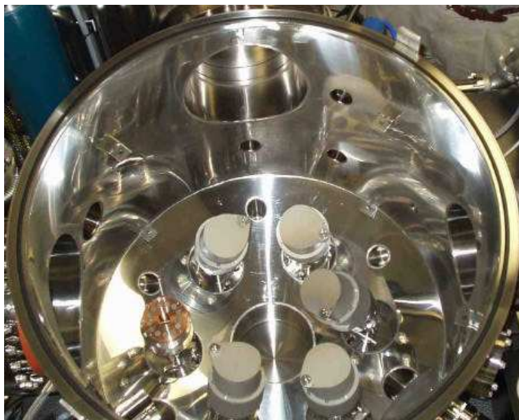
Figure 1.27: Photograph of the sputtering chamber showing six magnetron sources. Five of them are covered with a shutter, one is uncovered (on the left) showing the magnets within the source. The sources are at various tilt-angles.
