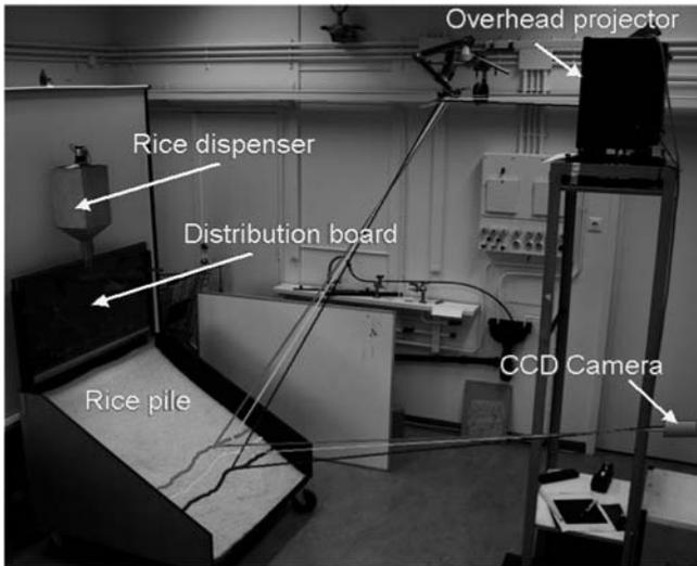
**Fig. 1.** The rice set-up with  $1 \times 1 \text{ m}^2$  floor area. Rice rains down from the distributor board onto the top of the pile. The 3-dimensional shape of the pile is reconstructed from the shape and position of a set of coloured lines projected onto the pile
