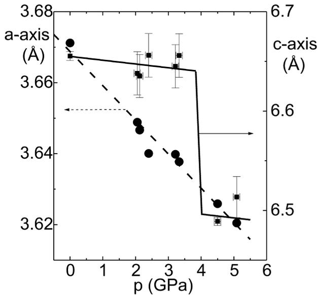
Fig. 4. Pressure dependence of the  $a$ - and  $c$ -lattice parameters of  $\text{YH}_3$ . A rearrangement of hydrogen atoms is probably responsible for the jump in  $c$  around 4 GPa.
