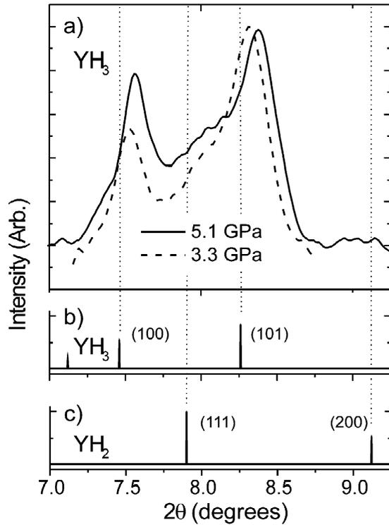
Fig. 3. (a) X-ray diffraction spectra obtained at the ESRF Synchrotron facility with 0.41345 Å radiation, above and below the high-pressure structural phase transition of  $\text{YH}_3$ . For comparison zero-pressure spectra for hcp  $\text{YH}_3$  (b) and for fcc  $\text{YH}_2$  (c) are also indicated. Clearly, both high-pressure spectra shown in (a) are consistent with a hexagonal phase as in (b) but not with a cubic phase as in (c).
